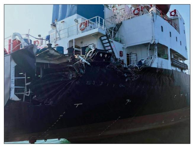
Figure 3: Damages sustained by DK Iman
